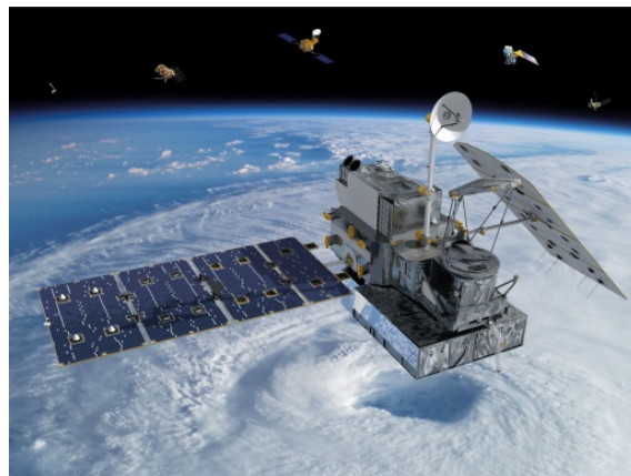
FIGURE 3.4.1 An artist's conception of the core observatory spacecraft of the Global Precipitation Measurement mission, a joint activity with NASA and the Japan Aerospace Exploration Agency. SOURCE: Courtesy of NASA.
